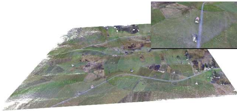
Fig. 9 The reconstructed point-cloud of the Rothenthurm area based on the combination of the RGB and grayscale camera data as well as the UAV pose estimates collected during the lawn-mowing path and subsequently processed using the Pix4D software.
