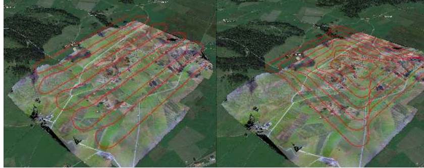
Fig. 8 The lawn-mowing path executed by the AtlantikSolar UAV overlaid on the reconstructed mosaic of the environment, incorporated in Google maps.
