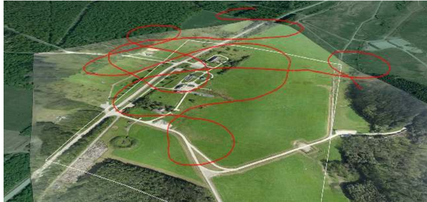
Fig. 6 Inspection path full area coverage using the oblique-view mounted thermal vision and grayscale cameras of the AtlantikSolar sensor pod. The colored mosaic was derived using an additional very large field of view nadir-facing camera (HDR-AS100VW).
