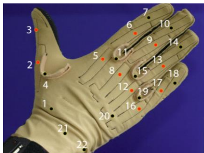
Fig. 2. CyberGlove II data-glove. The red dot represents our estimate of 10 angles
