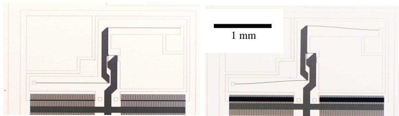
Figure 4. Microscope pictures of the undeflected and 100 \mu m deflected Watt's mechanism.
