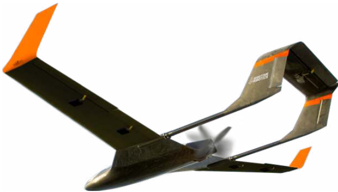
Fig. 7. P31016 concept battery-powered fixed-wing unmanned aircraft
