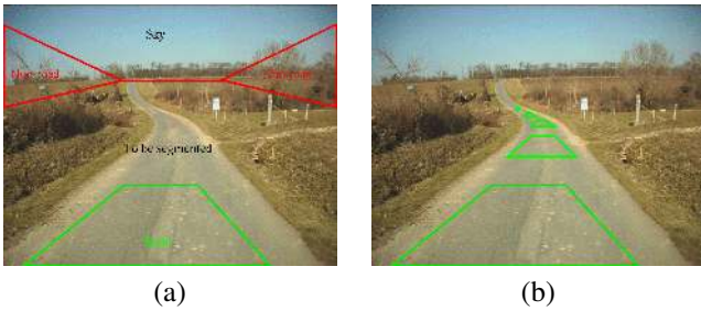
Fig. 2. Regions for road and non-road colors sampling on each image (a) and equivalent road regions for a sequence (b).
