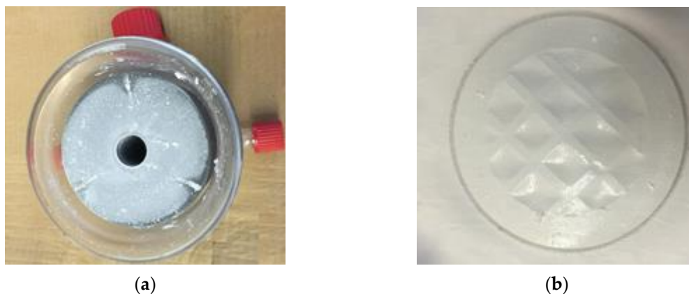
Figure 6. After the experiment with synthetic RO brine: (a) Membrane module; (b) Membrane surface. Salt crystals deposits are visible, which can easily be removed by washing with water.
