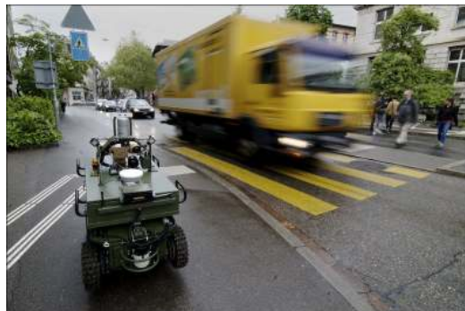
Fig. 1. ARTOR, a search and rescue robot specialized for outdoor applications navigating in a highly dynamic urban environment. Typical mobile elements include pedestrians, bikers, cars, trucks and trams.
