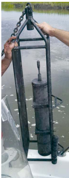
Fig. 2. Long-term acoustic recorders (DSG-Ocean) were deployed on the bottom of the May River. DSG-Ocean recorders in frames to minimize noise artifacts and impacts on the instruments
