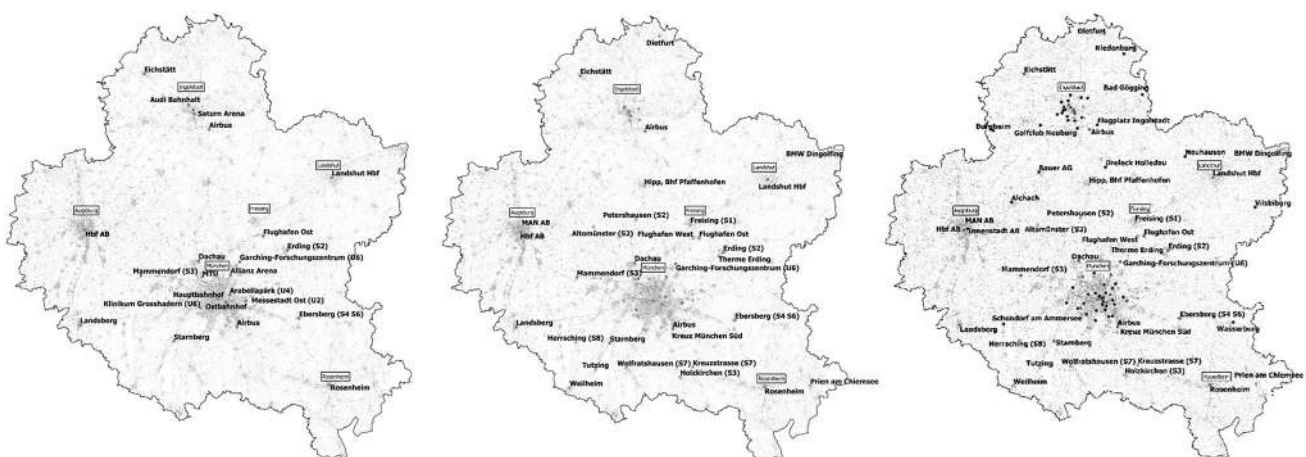
Fig. 6 Low (left), medium (middle) and high-density networks (right) for the study area with 24, 74 and 130 vertiports respectively [28]
