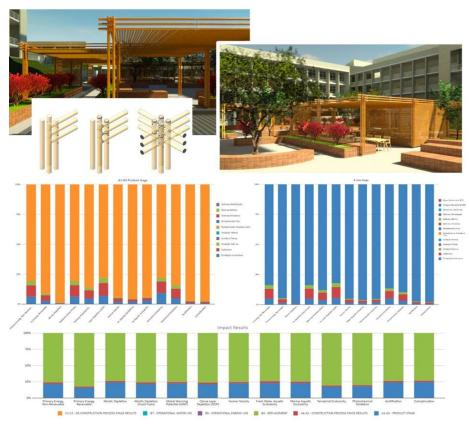
**Figure 7.** Illustrative excerpt of the circular design challenge hand-in board: LCA study for a bamboo and adobe structure. Image courtesy: Team B (2020). Original in Portuguese.
