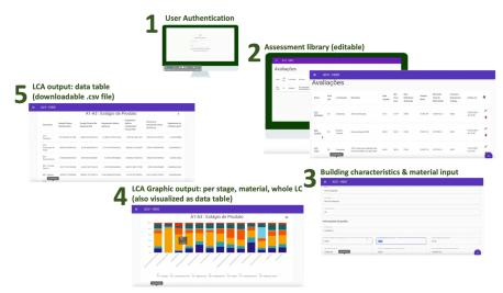
**Figure 11.** Online tool's interface (in Portuguese): information can be manually input or uploaded and edited as needed. Contribution analyses are broken down into building materials and subsystems, as well as per life cycle stage and for the complete cycle. The corresponding data table can be downloaded (.csv file) for detailed analysis.
