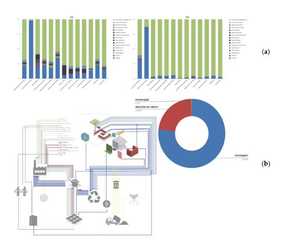
**Figure 9.** Illustrative excerpt of the circular design challenge hand-in board: LCA, system mapping, and identification of circularity bottlenecks for steel (LCA I) and for wood (LCA II) structural studies (**a**). System mapping ('50 years and 1 day') and material cycle closure indicator (blue lines on mapping) for refined LCA III (**b**), avoiding 77% of landfill disposal. Image courtesy: Team C (2019). Original in Portuguese.
