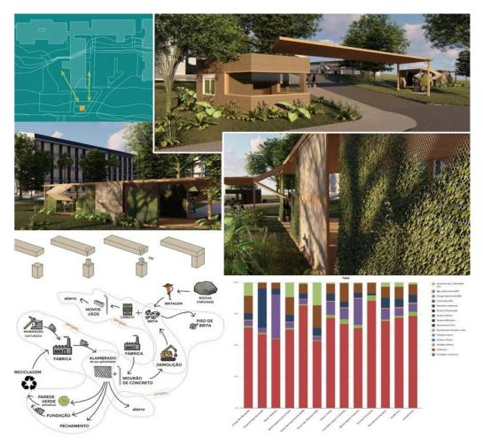
**Figure 6.** Illustrative excerpt of the circular design challenge hand-in board: urban equipment design, design logic for disassembly, system mapping and identification of circularity bottlenecks, and impact analysis through LCA. Image courtesy: Team A (2020). Original in Portuguese.
