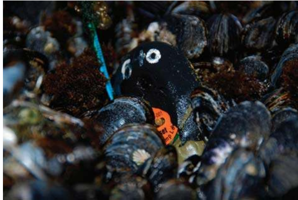
Figure 1. Epoxy ‘robomussel’ biomimetic logger (~8 cm in length) deployed in growth position in a Mytilus californianus bed. Loggers were designed to match the thermal characteristics of bivalves and were typically made of epoxy (as shown) but real shells filled with silicone were also used, especially for smaller (4 cm) mussels.
