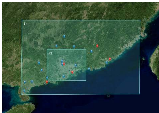
Fig. 5. Domains considered in the model simulations. The outer domain (1) has the size of 900 \text{ km} \times 600 \text{ km} with a 3 \text{ km} horizontal resolution and is centered at (23.5^\circ \text{ N}, 114^\circ \text{ E}) . The inner domain (2) provides a finer resolution of 1 \text{ km} and covers a 300 \text{ km} \times 300 \text{ km} area, with the center at (22.8^\circ \text{ N}, 113.5^\circ \text{ E}) . The red symbols represent the radar stations, and the blue symbols represent the lightning detection stations.
