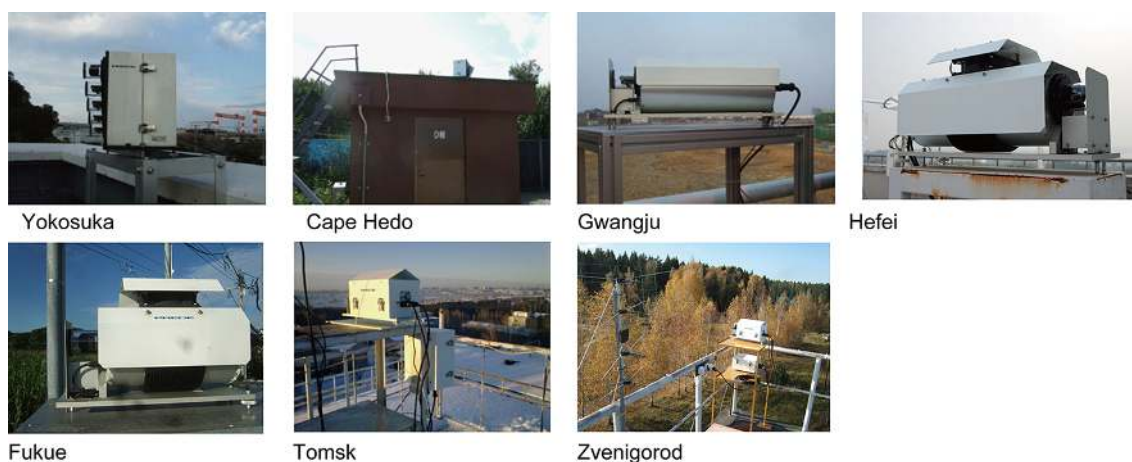
Figure 4. Light-receiving parts of MAX-DOAS instruments located at the seven sites.
