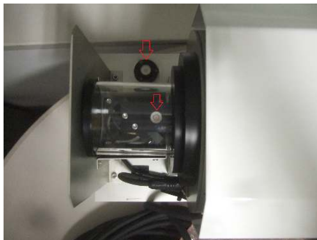
Figure 2. Two horizontal levels embedded in the base plate (upper arrow) and in a plate holding the reflecting mirror (lower arrow) were used to adjust the zero angle of the reflecting mirror.
