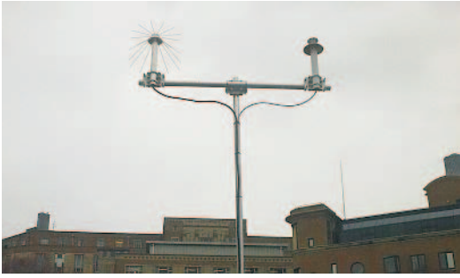
Fig. 1. Measurement antennas. The low band discone antenna is on the left, and the high band antenna can be seen on the right.
