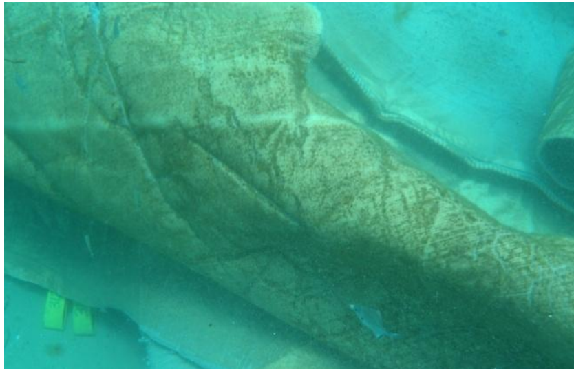
Figure 8. Failed container with polyurethane coating
