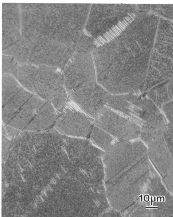
Figure 5f: Optical photomicrograph of alloy 706-3 exposed at 704°C for 5,000h.
