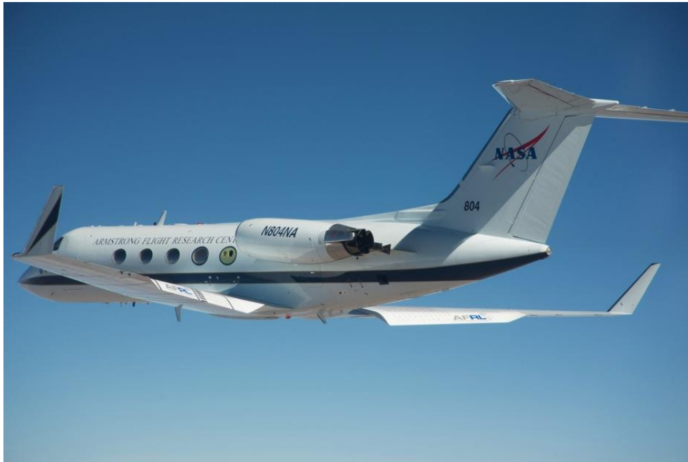
Figure 1. Test airplane in flight with ACTE flap deflection of 25 deg.
