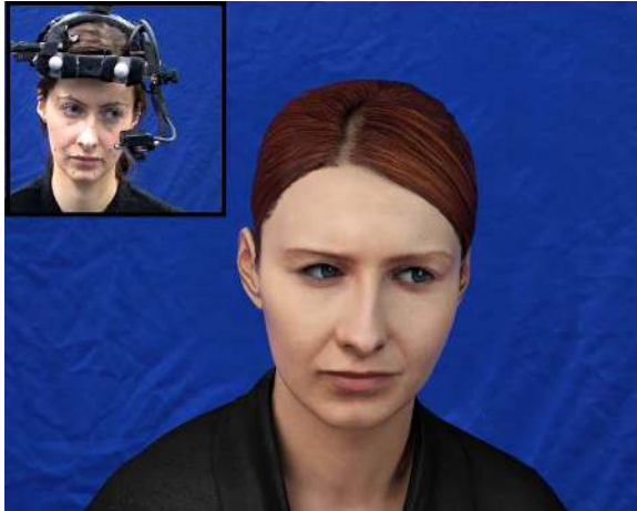
Figure 5: Eye movement capture using a head-mounted eye-tracking device, and corresponding virtual avatar displaying the recorded eye-movements [MBB12]
