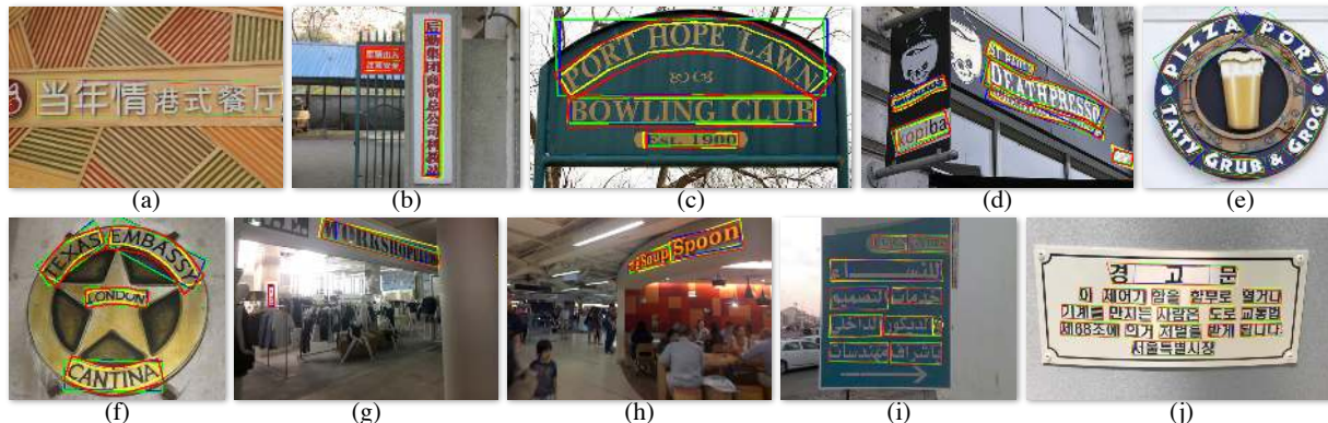
Figure 5. The visualization of detection results. (a) (b) are sampled from ICDAR2017-RCTW, (c) (d) are from SCUT-CTW1500, (e) (f) are from Total-Text, (g) (h) are from ICDAR2015, and (i) (j) are from ICDAR2017-MLT. The yellow polygons are ground truth annotations. The localization quadrangles in blue and in green represent the detection results of DR and IRM respectively. The contours in red are the detection results of SEM.
