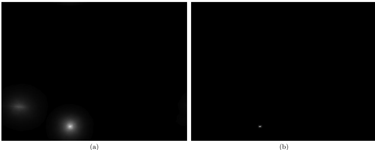
Figure 5: Illustrative Example G3: Filter Estimate \hat{X}_{3130} from: (a) Single Pixel Filter Bank and (b) Proposed Shape-Adaptive Filter Bank. The aircraft is the bright feature in both images. The bright feature on the left side of (a) is a cloud. As expected the aircraft estimate is more distinct in the shape-adaptive filter.
