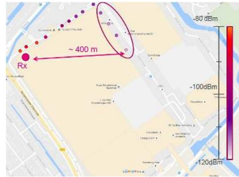
Fig. 4. The outdoor measurement locations and their RSSI values with SF 12.
