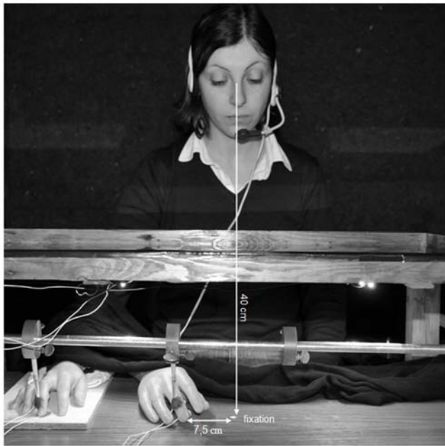
Figure 2. Set-up experiment 1. The picture represents an actor who consented to be photographed for illustrative graphical purposes. Viewing distance from the fixation point is reported, as well as the distance between the rubber hand middle finger and the fixation point (in cm).
