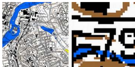
Fig. 1. Example of color map image: full size (left) 1024 \times 1024 pixels and (right) 100 \times 100 part.
