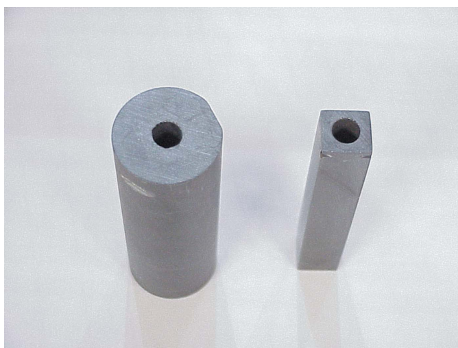
Figure 5 Photograph of the original and cut-down single-crystal silicon sample holders. Left: 25 mm-diameter full cylinder (mass of 80.68 g) with 6.5 mm drilled hole. Right: 11.2 × 11.8 mm silicon holder with 6.5 mm drilled hole trimmed from circular to square cross section (mass of 18.33 g). Notches near the top allow for mounting onto sample bases using set-screws. Teflon tape is normally wrapped around the silicon at notch level so as to avoid local stresses due to the set-screws.
