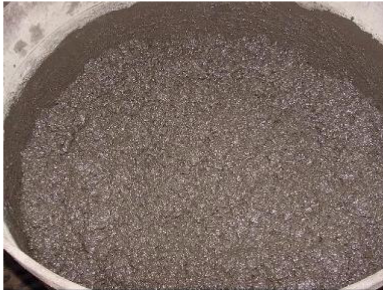
Figure 3.4 Fresh Geopolymer Concrete
