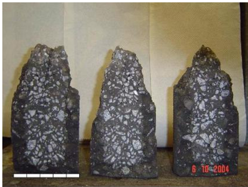
Figure 4.44 Damage to Test Cylinders Exposed to 2% Sulfuric Acid Solution
