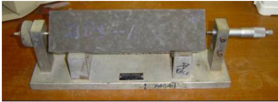
Figure 3.16 Horizontal Length Comparator with Drying Shrinkage Test Specimen
