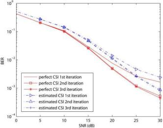
Fig. 10. BER performance of equalizer II/III under channel estimation uncertainties.
