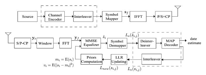
Fig. 1. System model for the proposed block turbo equalizers.
