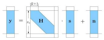
Fig. 2. System input-output relation after removing the guard intervals.
