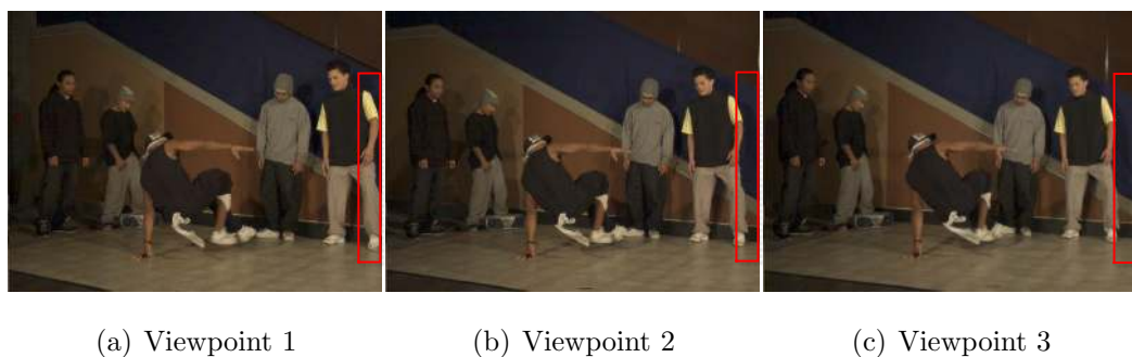
Figure 1.3: An example of multiview video: frames from the Breakdancers sequence depicting a scene from three different viewpoints. The horizontal offsets between the three viewpoints can be clearly observed in the portions of the frames identified by the red rectangles.
