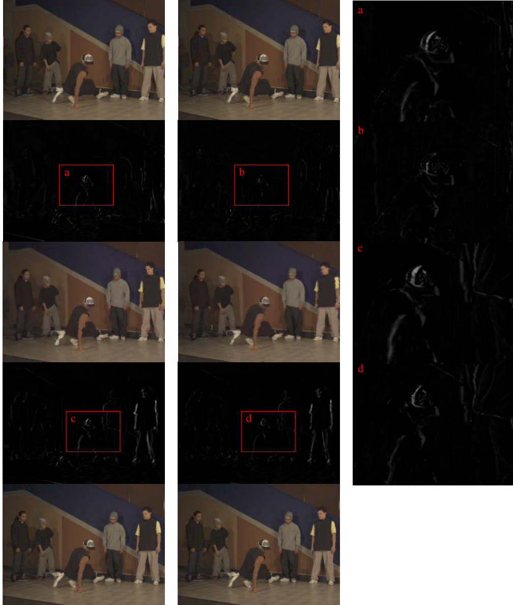
Figure 5.9: Comparison of Inter-view Consistency. Left: baseline method, Centre: proposed method, Right: Zoomed difference images. The first two columns show (from top to bottom): the frame F_{v-,t} , the difference of the warped frame from F_{v,t} to F_{v-,t} and the frame F_{v-,t} , the reconstructed frame F_{v,t} , the difference of the warped frame from F_{v,t} to F_{v+,t} and the frame F_{v+,t} , and the frame F_{v+,t} respectively. The third column shows the zoomed difference images from the first two rows. For these results, a frame in view 1 of the Breakdancer sequence was dropped and then concealed using the baseline BMA and the proposed method. The zoomed parts of the difference images show higher inter-view consistency (smaller magnitude of the white color) of the proposed method compared to the baseline BMA method.
