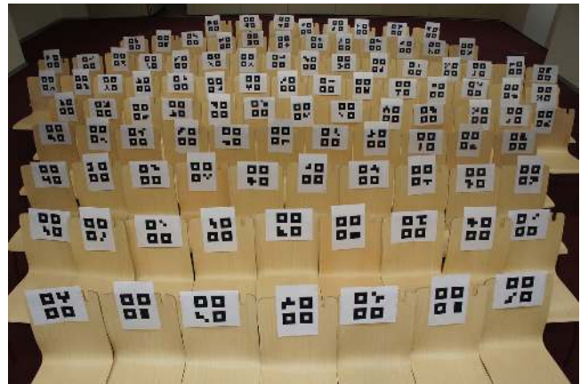
Figure 5: A simulated 100-person classroom. Our algorithm recognizes all 100 qCards in under 5 seconds from a webcam video stream, or in 85ms from this high-quality still image.
