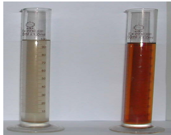
Fig. 11. Left: treated raw water; Right: untreated raw water
