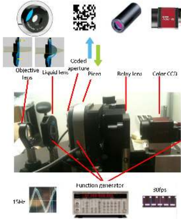
Figure 4. Setup of the camera.
