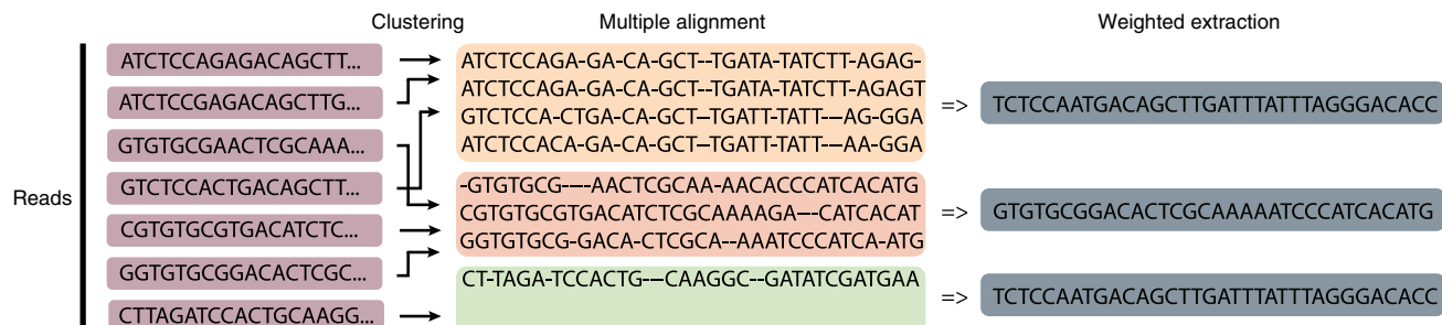
Fig. 5 Clustering and extraction of read DNA sequences. The sequenced DNA fragments are clustered, aligned and possible candidates are extracted in a majority voting step. The alignment is visually enhanced by marking deletion errors with a dash.
