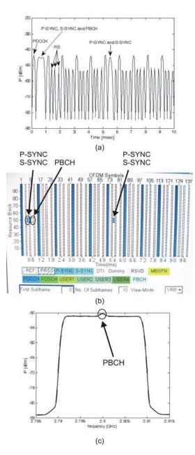
Once the PBCH power is measured with these correct SA settings, the following method is proposed to estimate the maximal exposure level ( $E_{max}$ ) of the LTE signal at a measurement location (the extrapolation method is valid for both SISO and MIMO):
