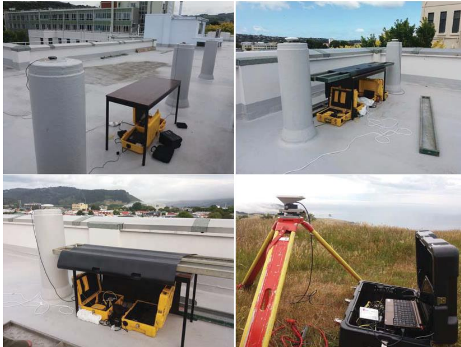
105 106 Fig. 1 GNSS ublox EVK-M8T receivers collecting data for GPS + BDS single-baseline RTK, with 107 patch antennas (top, left) and Trimble Zephyr 2 antennas (top, right) in Jan 4-6 and Jan 6-8, 2016, 108 respectively. Survey-grade Trimble NetRS dual-frequency GPS receivers have been connected to 109 the same Zephyr 2 antennas to truly track the same GPS constellation. A 7 km baseline setup (Jan 110 18-19, 2016) also used to assess the positioning performance is shown at bottom 111
