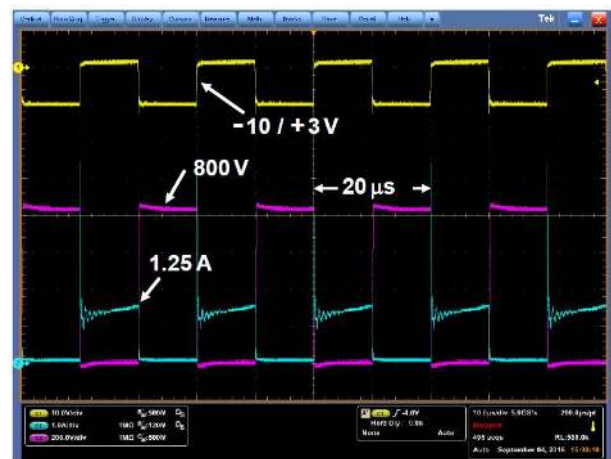
Figure 13 Hard-switching characteristics of the 400V-800V boost converter using PSJ-FETs. The red line shows the drain current and the blue line shows the inductor current.
