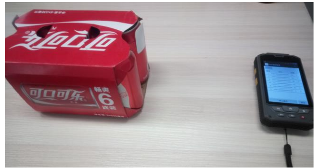
Fig. 20. Read range measurement of half dozen pack of metallic can
