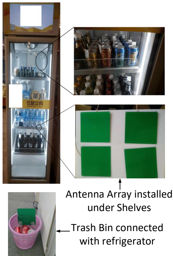
Fig. 23. Commercial testing set up in operation for a metallic can with RFID
