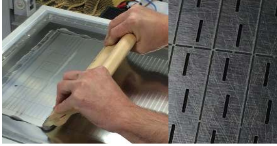
Fig. 9. The soldering paste is set in place manually with the aid of a stencil. The picture to the right shows the outcome of the process. The black lines framing the slots is the deposited paste.
