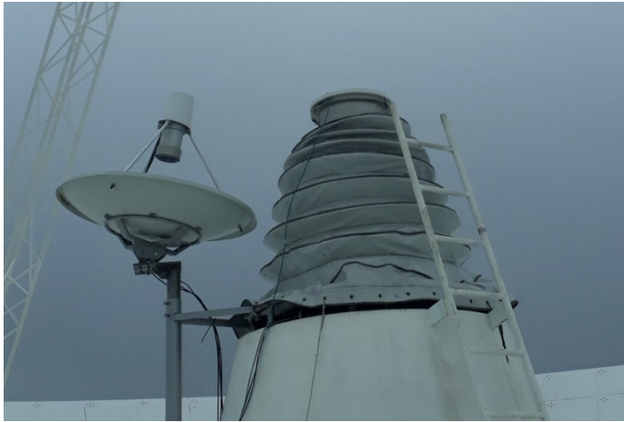
Fig. 4. L-band feed antenna installed at RT-32 with offset from secondary focus.
