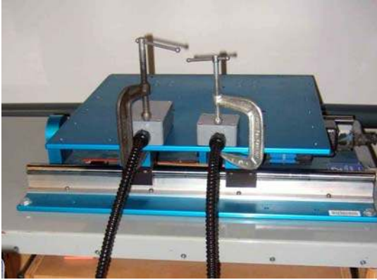
Figure 5-39: Horizontal shake device with two accelerometers attached.
