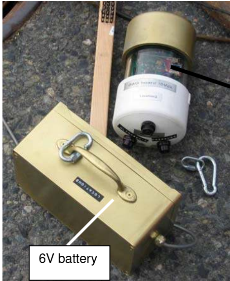
Figure 4-6: Intel Mote + Data Acquisition Board and Battery packaging
