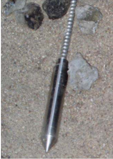
Figure 5-1: Steel housing from previous experiment (Aw 2004).
