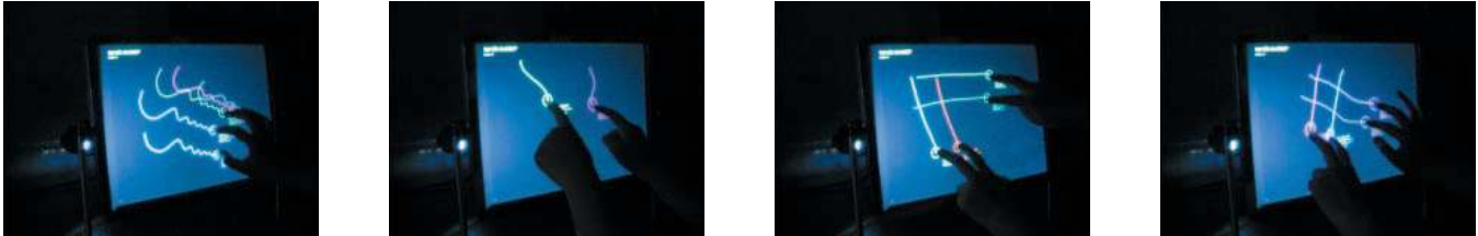
Figure 1: Simple examples of multi-touch interaction using our FTIR technique
