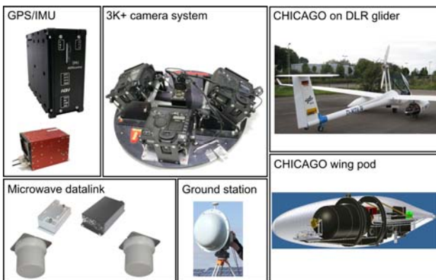
Figure 2. Airborne hardware components and data flow of the 3K camera system for the real time processing chain
