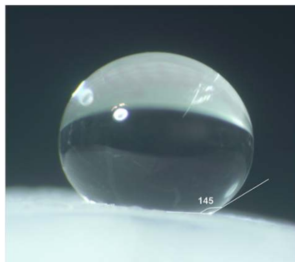
Fig. 2. Contact angle photograph of water droplet on hydrophobic surface of silica aerogel.
