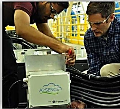
Figure 73. AirSENCE devices installed on TTC streetcars for monitoring ozone, carbon monoxide, carbon dioxide, and PM 2.5 along King Street routes 11 .
