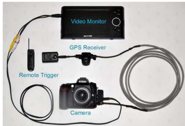
Fig. 3 Connections among four components (camera, GPS, monitor, and remote trigger) of an imaging system.
