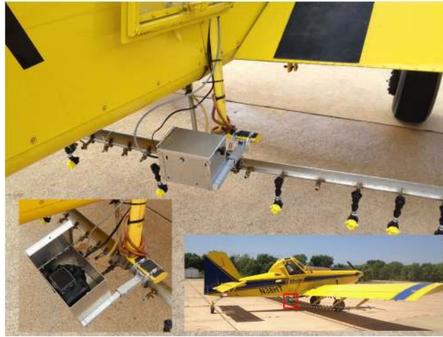
Fig. 2 A Nikon camera mounted on the right step of an Air Tractor AT-402B. A GPS receiver and a video monitor integrated with the camera are mounted in the cockpit.
