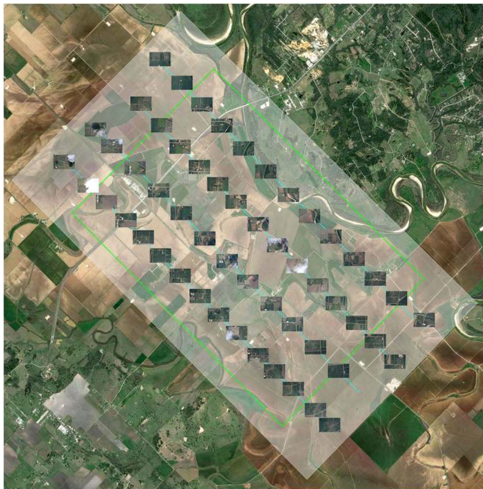
Fig. 7 Geotagged images plotted in Google Earth. The images were acquired at 1524 m (5000 ft) above ground level near College Station, Texas.
