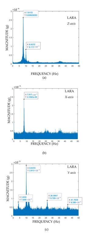
**Figure 12.** Eigenfrequency analysis of a footbridge using LARA for (**a**) vertical, (**b**) longitudinal, and (**c**) transversal directions of the footbridge.
