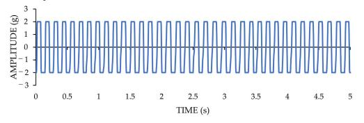
Figure 9. The time-domain presentation of acceleration amplitude saturation of LARA.
