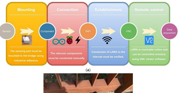
the diagram of LARA setup on the bridge. The location of the commercial dynamic sensor (HI-INC) and LARA on the mid-span of the bridge is shown in Figure 11b.
