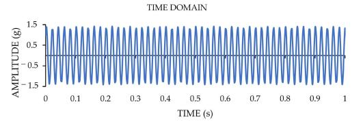
Figure 8. The time-domain presentation of a vibration acquisition with RMS value of one g by LARA.
