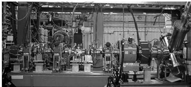
Figure 1: This picture shows the assembled HEBT including magnetic transport elements (i.e., four quadrupole and two steering magnets) and beam instrumentation.
