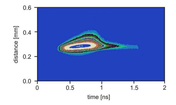
Pinhole + X-ray Streak Camera 1024x400 pixels, x: 3.3 ps/pixel, y: 2.0  $\mu$ m/pixel filters (1 mm Be, 8.5  $\mu$ m aluminized mylar)  $\rightarrow E_{ph} > 2.5 \text{ keV}$ 3 $\omega$  experiments (50-250 J, 0.44  $\mu$ m, 250 ps, 0.4–2×10<sup>16</sup> Wcm<sup>-2</sup>): limited duration and spatial extent of the plasma emission
