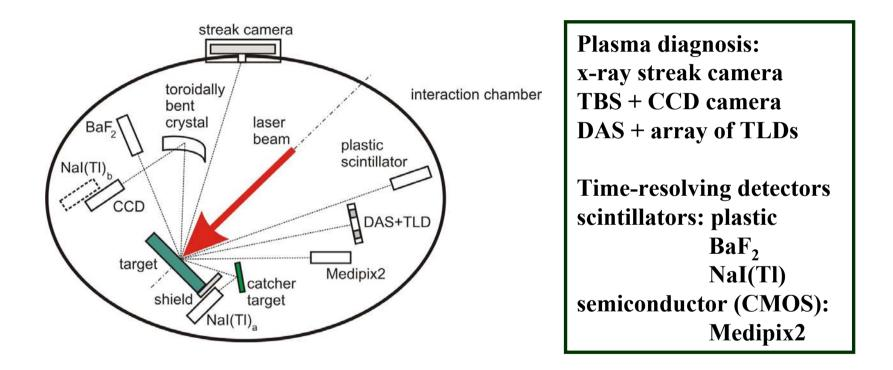
Prague Iodine Laser System PALS single Gaussian-profile beam (1000 J/1 $\omega$ , 1.315  $\mu$ m, 0.3 ns, 80  $\mu$ m, 7×10<sup>16</sup> Wcm<sup>-2</sup>) frequency-tripled radiation (300 J/3 $\omega$ , 0.44  $\mu$ m, pulse length 0.25-0.3 ns)
