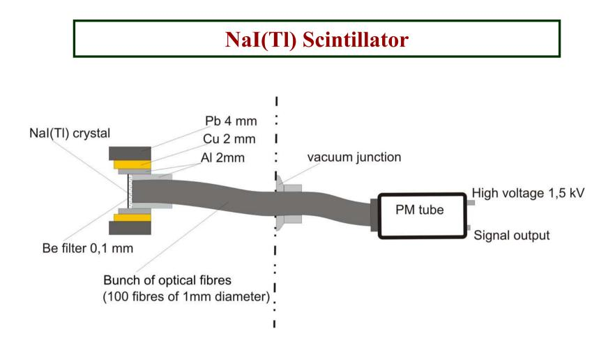
NaI(Tl) scintillator (diameter 25 mm, thickness 1 mm)
