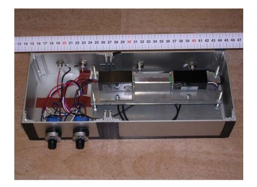
plastic and BaF<sub>2</sub> scintillation crystals, active size  $4 \times 8 \times 65 \text{ mm}^3$ ,  $3 \times 10^{-3}$  srad glued to two fast photomultipliers operating in a coincidence mode LeCroy oscilloscope WavePro7000 (band width 1 GHz, sampling rate 1 GS/s) duration of the fast signals shorter than 5 ns calibrated using <sup>55</sup>Fe (5.9 keV) and <sup>241</sup>Am emitters (~60 keV)
