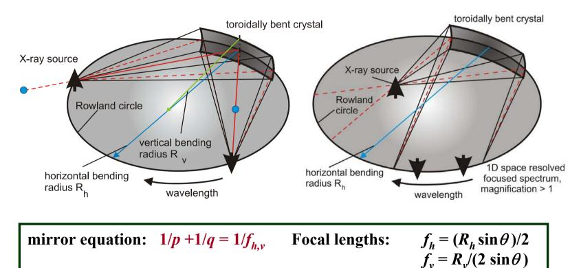
spectroscopic application:  $\Delta\lambda$  coverage requires source inside RC spectra dispersed onto detector positioned at Rowland circle combination of spectral and 1D spatial resolution
