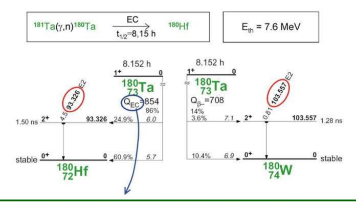
Transmutation of <sup>181</sup>Ta (γ, n) to <sup>180</sup>Ta and further to stable <sup>180</sup>Hf (probability 86%) or <sup>180</sup>W (probability 14%) accompanied by weak γ emission at 93.3 keV (Hf) or 103.5 keV (W) and strong x-ray Hf Kα<sub>1</sub> (55.8 keV), Kα<sub>2</sub> (54.6 keV) and Kβ (63.2 keV) emission due to numerous holes in K-shell of Hf → identification of Ta decay
