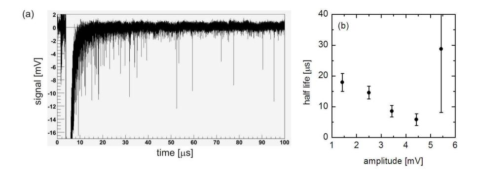
Detector calibration using the <sup>55</sup>Fe radionuclide → signal amplitudes corresponding to decay of nuclei <sup>181</sup>Ta expected at level of 1-2 mV Alternate half-lives for different pulse amplitudes do not allow univocal interpretation of the measured signals
