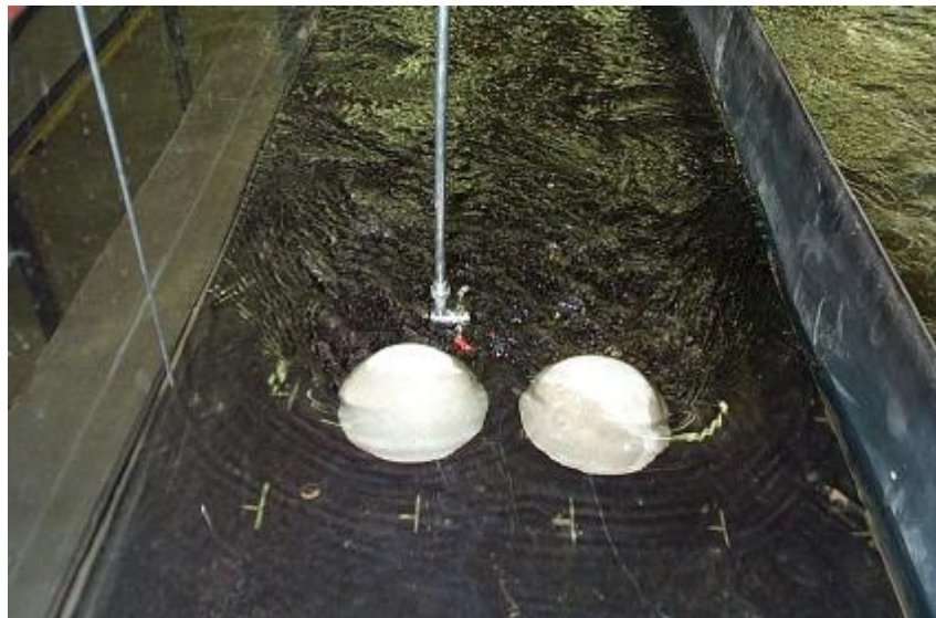
Figure 5-2 Tests 1, two hemispheres with spacing of 0.14 m
