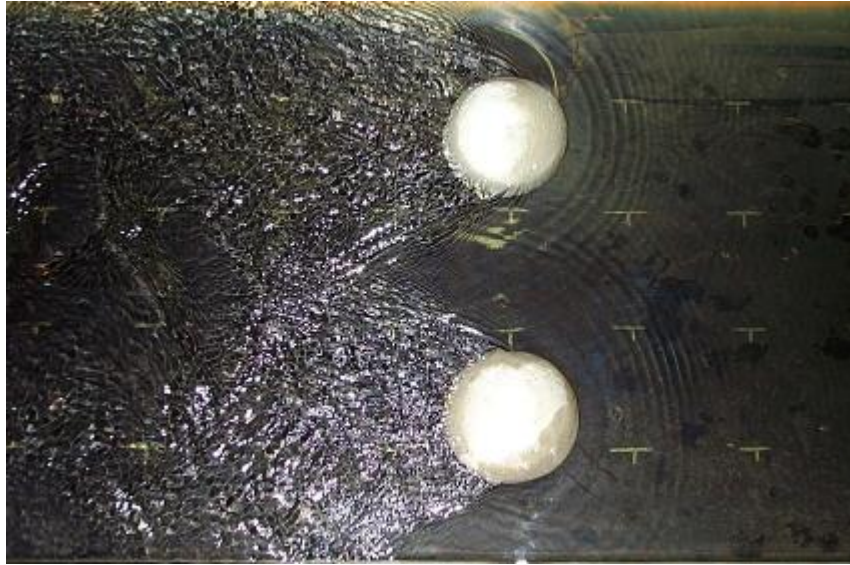
Figure 5-4 Test 2, two hemispheres with spacing of 0.24 m
