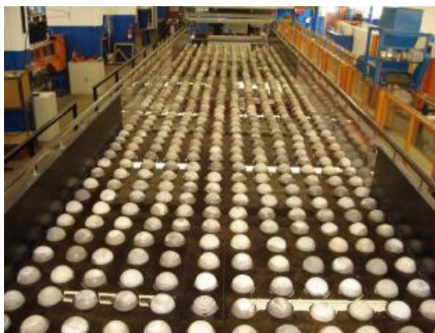
Figure C-17 Pattern 17 - H1 spacing cross-sectional 0.110m, longitudinal 0.167m
