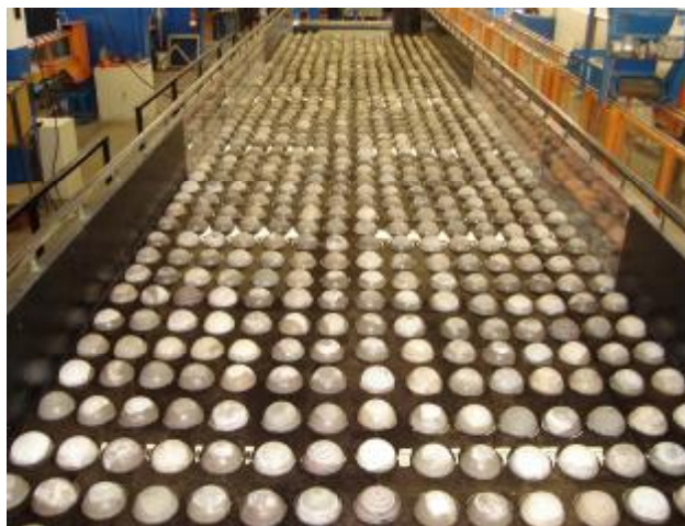
Figure C-16 Pattern 16 - H1 spacing cross-sectional 0.110m, longitudinal 0.125m
