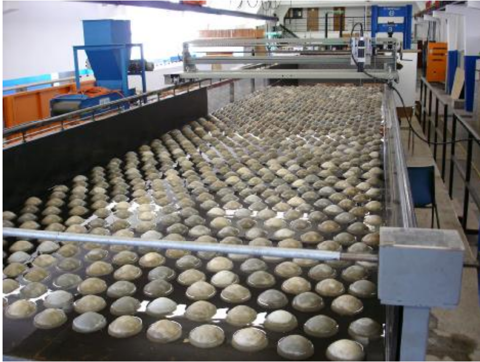
Figure 3-5 Flume C with a staggered pattern of hemispheres
