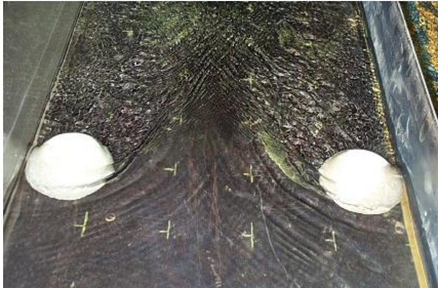
Figure 5-6 Test 3, hemispheres with spacing of 0.38 m
