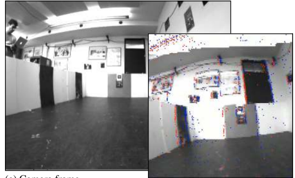
(a) Camera frame (b) DVS events + grayscale from camera Fig. 1. We present a visual odometry algorithm that uses low-latency brightness change events from a Dynamic Vision Sensor (DVS) and the data from a normal camera to provide the absolute brightness values.
