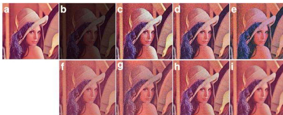
Fig. 7 Comparative results using simulated low-light image with \sigma = 15 : a input image, b simulated low-light image, c Chen's method [2], d Kim's method [3], e Jiang's method [8], f Ravi's method [23], g Jobson's method [14], h Fu's method [16], and i the proposed method ( \lambda_1 = 300 , \lambda_2 = 0.2 , \lambda_3 = 0.9 , and \omega = 10 )
