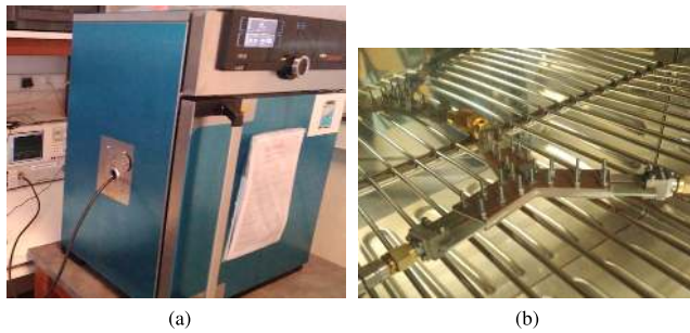
FIGURE 13. Temperature Test. (a) Union of the oven and the analyzer (b) Circulator inside the oven.
